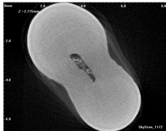
Inter-slice artefacts and odd shape in root canal
